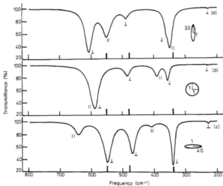
Figure 3. Calculated transmission spectra corresponding to three different particle shapes; (a) long prolate with  $L_{\perp} = 0.45$  and  $L_{\parallel} = 0.10$ ; (b) sphere with  $L_{\perp} = L_{\parallel} = \frac{1}{2}$ ; (c) the flat oblate with  $L_{\perp} = 0.15$  and  $L_{\parallel} = 0.70$ . Thick vertical bars on the abscissae indicate the observed peak frequencies.
